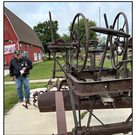
Chauncey Muedeking remembers how this horse-drawn grader was used to maintain township roads.
